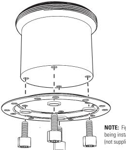
**NOTE:** Figure 2 shows the power module being installed on a PXM100 pedestal mount (not supplied).
